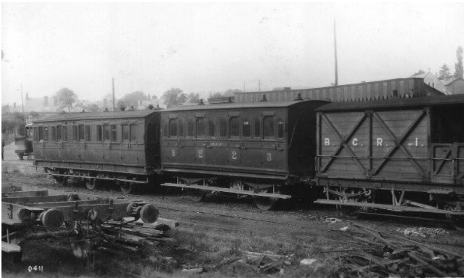
Bishop's Castle, 1928: the two coaches, both bought from the GWR, are, left, L&SWR built c.1885, (via the Brecon & Merthyr) tri-compo brake six-wheel coach, right an ex-Brecon & Merthyr four-wheel coach; and ex-GWR brake van no. 1, built post 1882. Note the variegated platform canopy, the town of Bishop's Castle beyond, and the evidence of DIY in the foreground.
