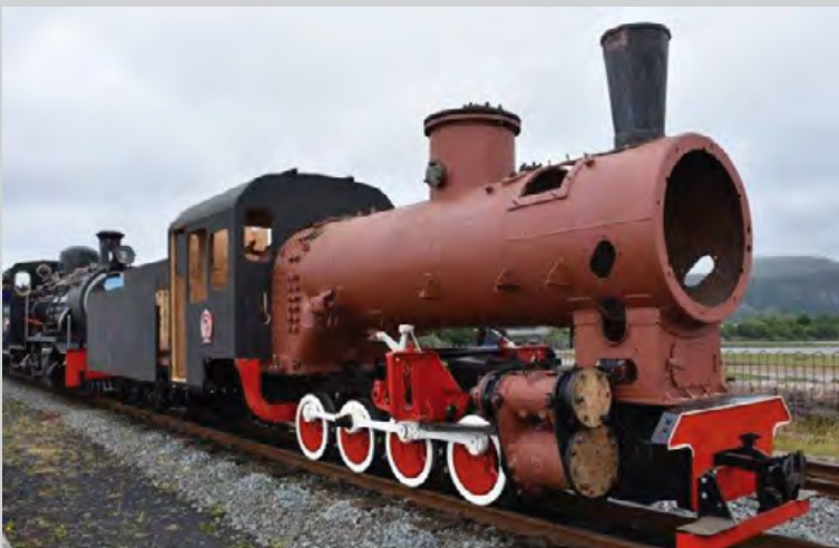
Bringing up the end of the cavalcade hauled by 134 was Harbin C2 class 0-8-0, Dahulichang no.4 which is currently being rebuilt for future service, probably on the WHR.
