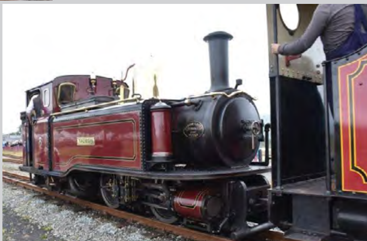
Single Fairlie Taliesin which was built at Boston Lodge in 1999 replicating the original 1876 locomotive which was withdrawn in 1932 and eventually scrapped.
