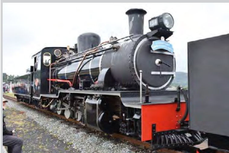
The newest locomotive to enter service is the Welsh Highland's former South African NG15 134, a 2-8-2 built by Société Anglo-Franco-Belge in 1952. Restored at the WHR's Dinas Works, it entered service in 2024.
