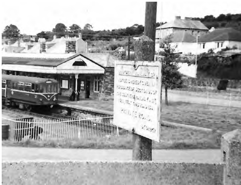
Bodmin North: AC Cars railbus W79978, waiting its booked departure back down the bank to Boscarne Exchange Platform. Hogging the shot is a Southern Railways cast sign on an Exmouth Junction concrete post behind a concrete fence.
