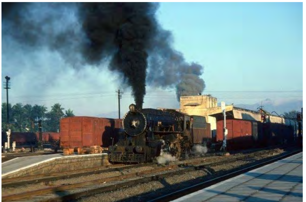
With the Nilgiri Hills in the background, broad gauge pilot at Coimbatore on 7th January was AWC 2-8-0 No.22615 (Baldwin, 1944) - essentially a 5'6" gauge USATC S160.
