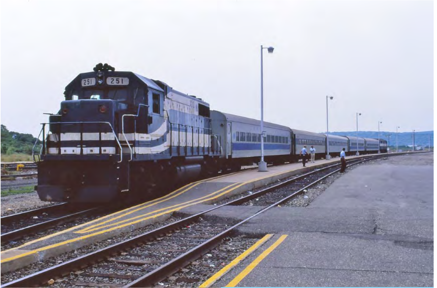
East end Diesel services were worked by these EMD GP38-2 2000hp locomotives represented by 251 at Montauk on 16th August 1985. When operating push-pull the locomotive would be found on the east or country end of the train.
