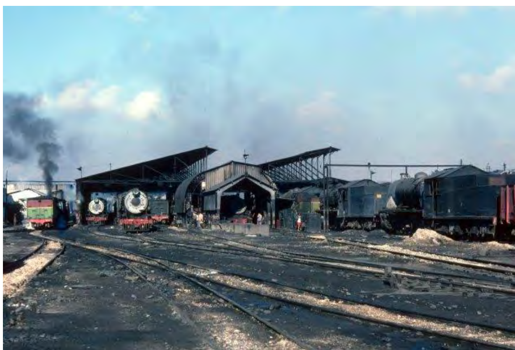
A general shed scene at Lallaguda in Secunderabad with, straight ahead, the metre gauge tracks containing various YP 4-6-2s and YG 2-8-2s and, on the right, the broad gauge tracks with two withdrawn XD 2-8-2s either side of an XB 4-6-2. Not a good photo, but this the only dual gauge shed visited
