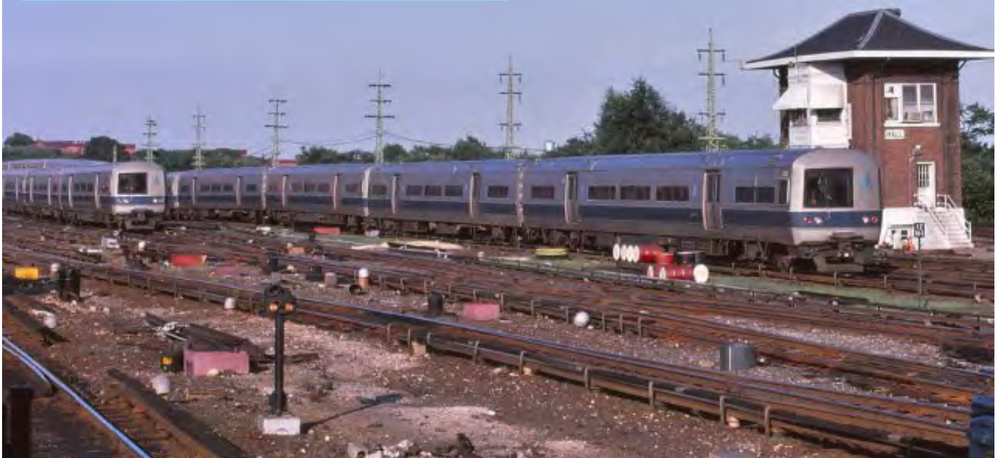
LIRR 'Metropolitan' EMUs passing Hall Tower at Jamiaca on 5th July 1987. Formed in 2-car sets, 770 cars designated M1 were built by Budd from 1968 followed by 174 M3s (seen here) with minor differences from 1985. All the M1s have been retired and the M3s are currently being retired.
