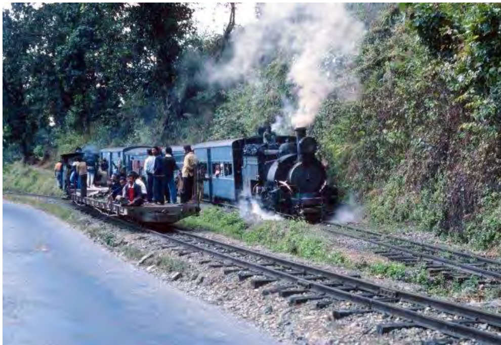
NFR 2' gauge B 0-4-2ST No.782 (Sharp Stewart 4562/99) on a down-hill works train passing No.783 (Sharp Stewart 4562/99) with Train ID, the 07:10 New Jalpaiguri to Darjeeling on First Reverse below Tindharia on 1st January 1980.
