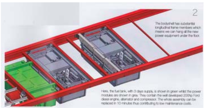
The fully enclosed engine/alternator units incorporating 5-cylinder Ford Transit diesel engines. Viva Rail
