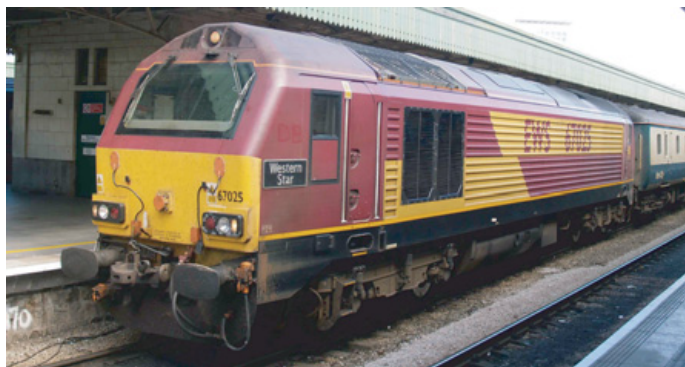
67025 Western Star on a FGW service at Cardiff Central on 19th August 2009. This is the no.2 end with the cooler group.
