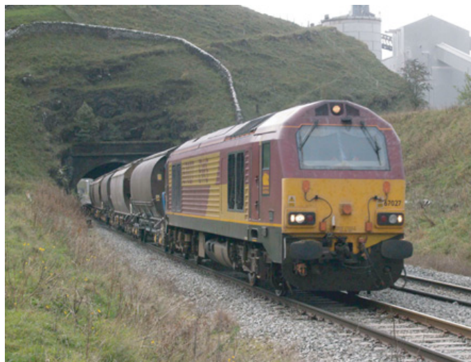
67027 Rising Star on a rare freight working at Great Rocks on 26th October 2006. This is also the no.2 end but shows the other side with the central air intake at the far end.
